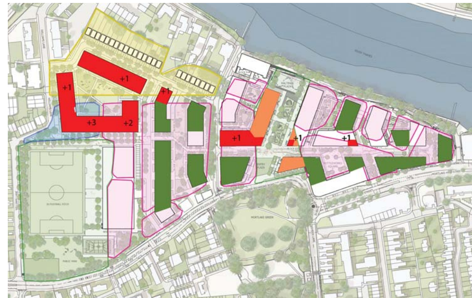
ORIGINAL PROPOSAL: COMPARISON OF HEIGHTS WITH PLANNING BRIEF (RED ABOVE & GREEN BELOW MAXIMUM HEIGHTS INDICATED IN PLANNING BRIEF)
