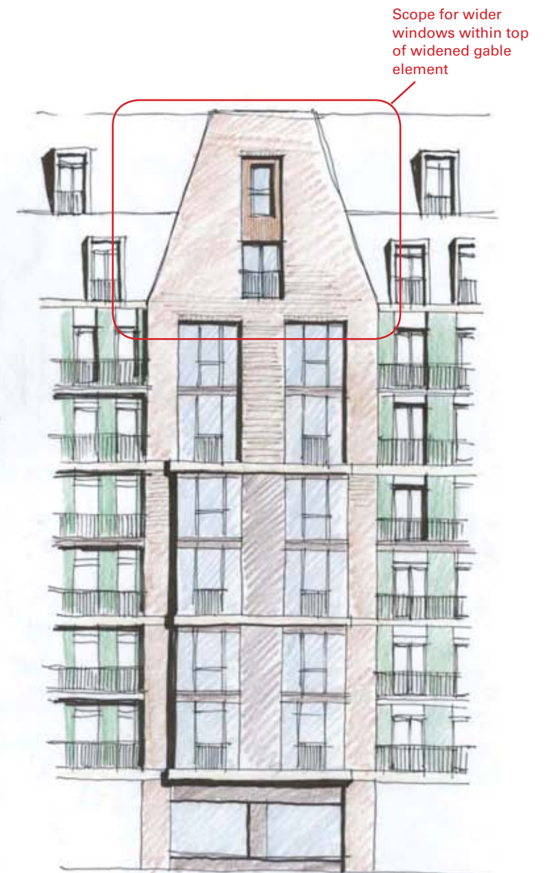
Widened 9 storey elevation
