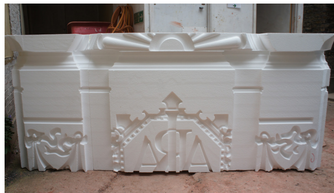
CNC cutting of polystyrene framework:
