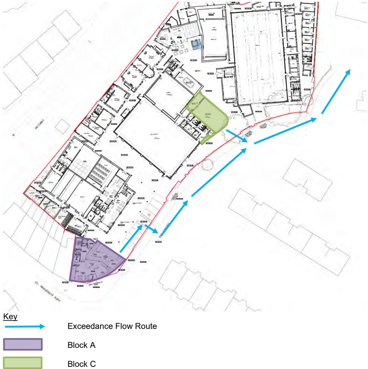
Figure 6: Exceedance Flood Flow Routing
