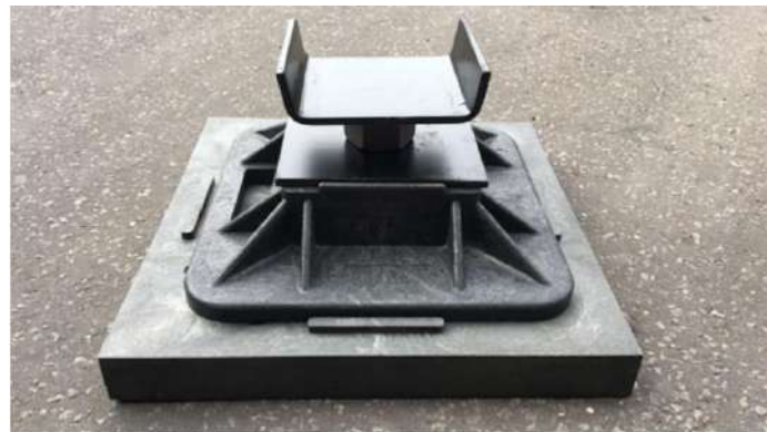
Single Jackpad footing, 450 x 450mm on plan, minimum 200mm tall. Based on an assumed spacing of 1000mm, should a wider spacing be preferred the ground will need to be verified for a suitable bearing capacity.
