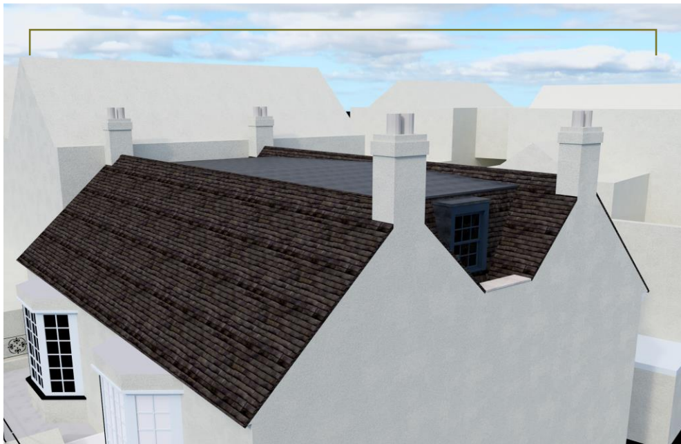
CGI visualisation of proposed scheme showing the set back roof infill preserving the existing roof form
