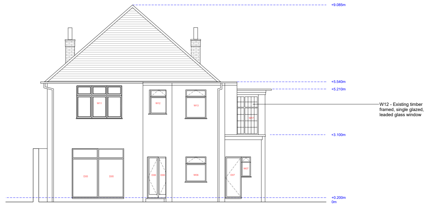
E3 EXISTING REAR ELEVATION 1:100
