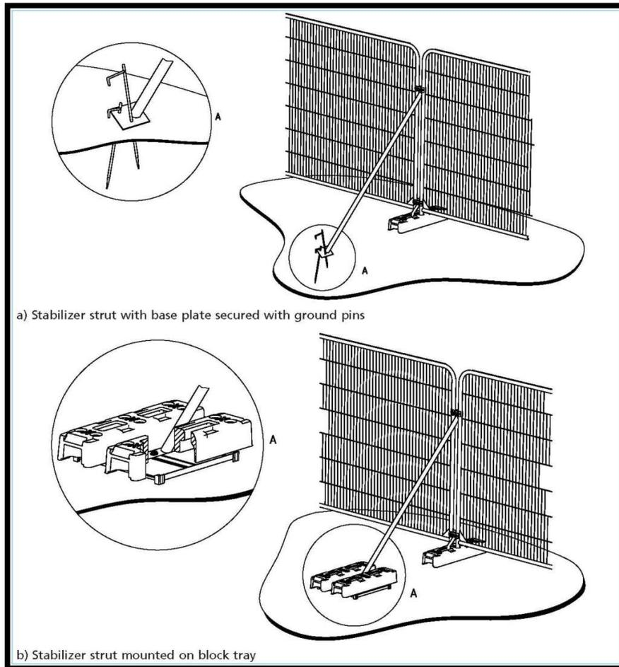
**Figure 3: BS5837:2012 - Figure 3, Examples of above-ground stabilising systems.**
