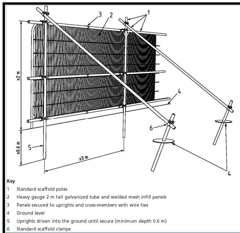
**Figure 2: BS5837:2012 - Figure 2, Default specification for protective barriers.**
