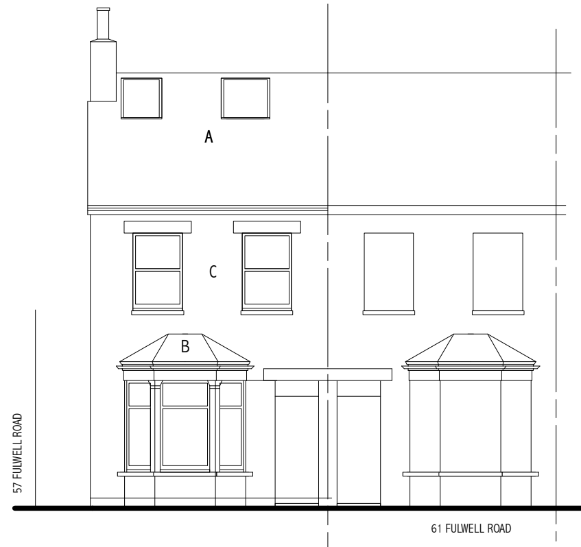
FRONT : NORTH ELEVATION PROPOSED - FACING FULWELL ROAD - 1:100 SCALE - NO CHANGE FROM EXISTING
