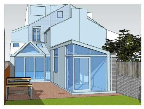
Externally the building will have just one new window and a set of sliding doors, finished in dark grey aluminium. New gutters and downpipes will be in black upvc. The solid walls will be of stock brickwork to match the existing house. The pitched roof will be in blue/grey artificial slate and the small area of flat roof will be in dark grey single layer high performance felt. The illustration below shows the view from the adjoining garden at No 33
