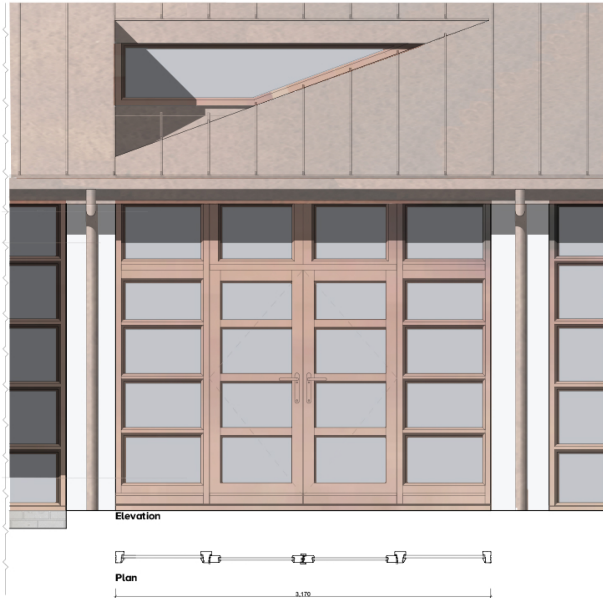
Timber double glazed conservation outward opening doors with side lights A1@1:20
