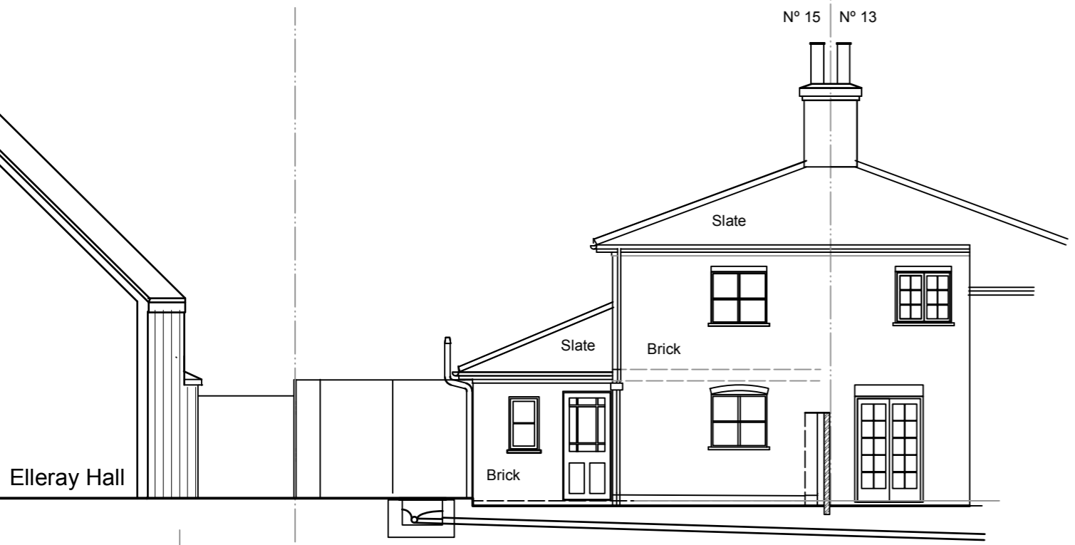
EXISTING REAR ELEVATION
