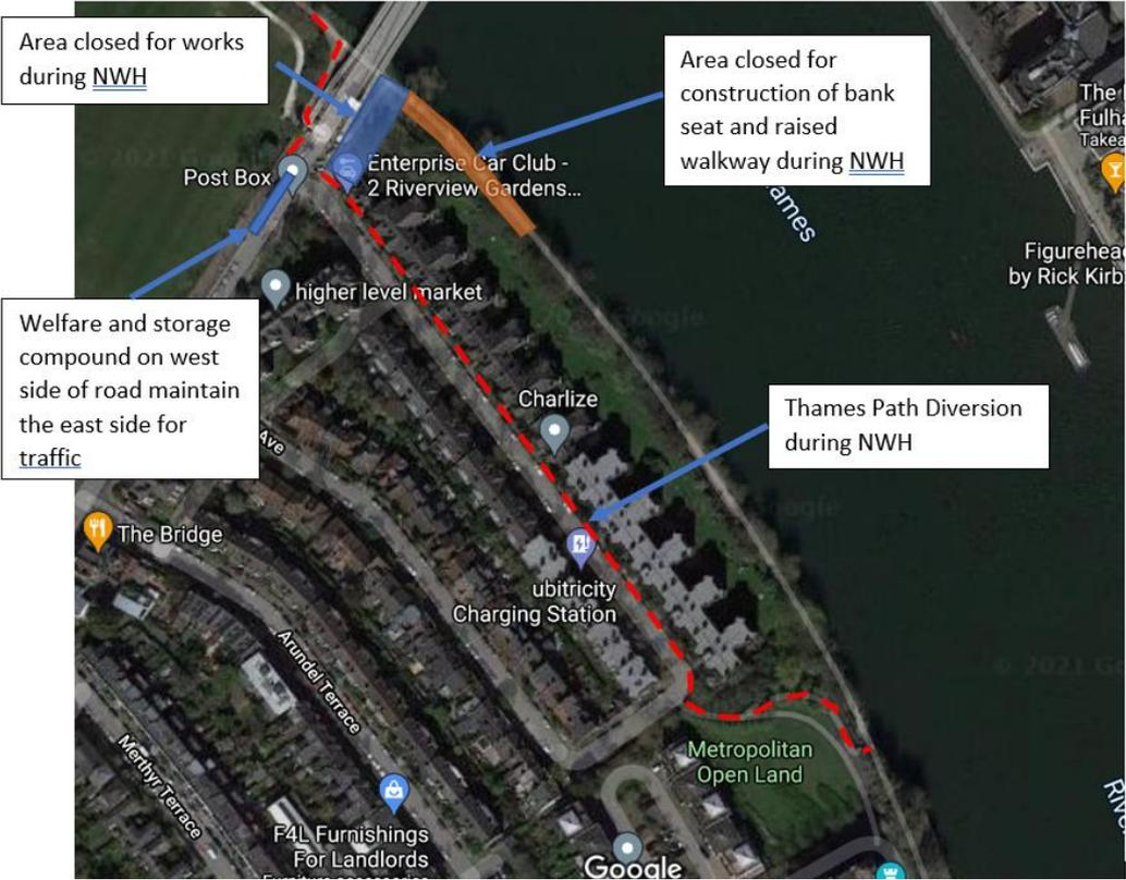
Figure 15 – Footpath Closure on south side of Hammersmith Bridge
