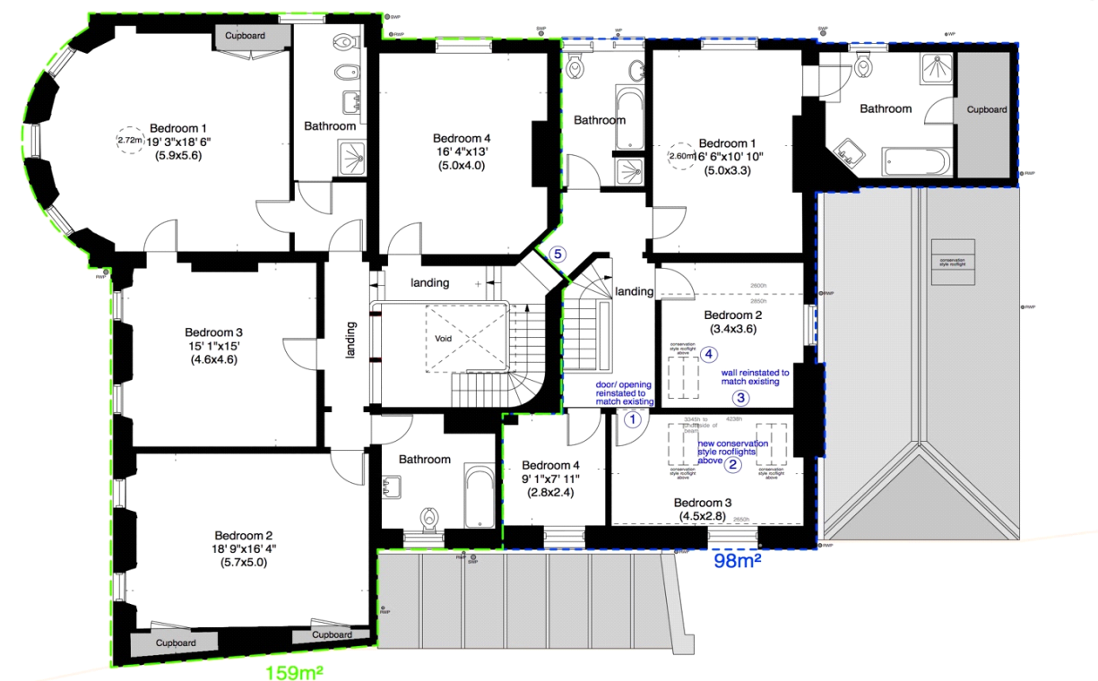
Fig. 22: First-floor plan of Riverside House and No. 1A Riverside, showing scope of proposed alterations, including reinstatement of features, and installation of roof-lights (approximate scale 1:200) (GPS Architecture).
