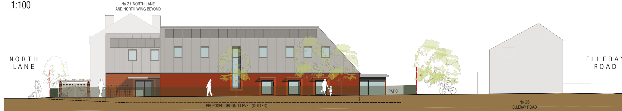
SIDE ELEVATION (SOUTH FACADE) 1:100
