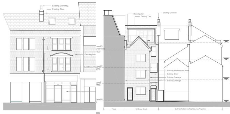
Figure 4. Front and Rear Elevations as Existing
