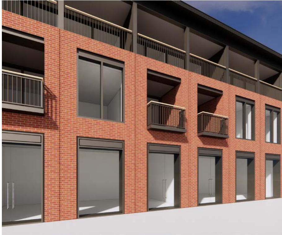
We looked at using the balcony to create a deep brick reveal that accentuated the contrast with the windows. We then pulled out the balconies to create more modulation of the facade
