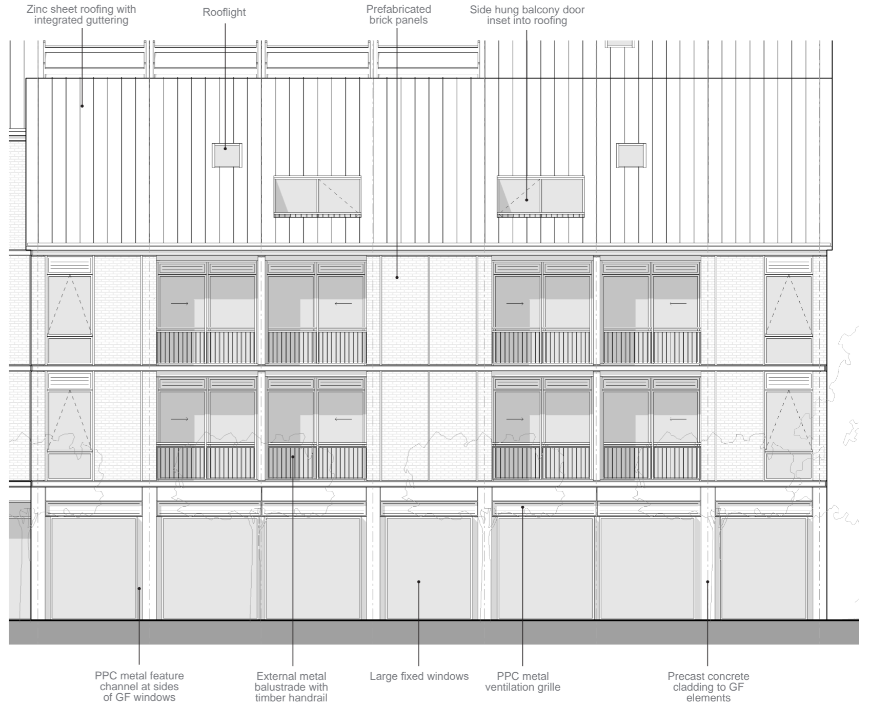
East Elevation - East Block
