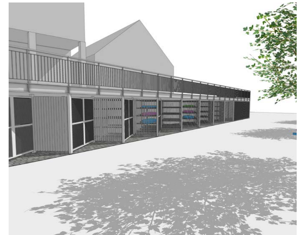
The doors to the individual boathouse sections have a lightly different façade treatment made up of PPC metal bars with gaps to allow water flow
