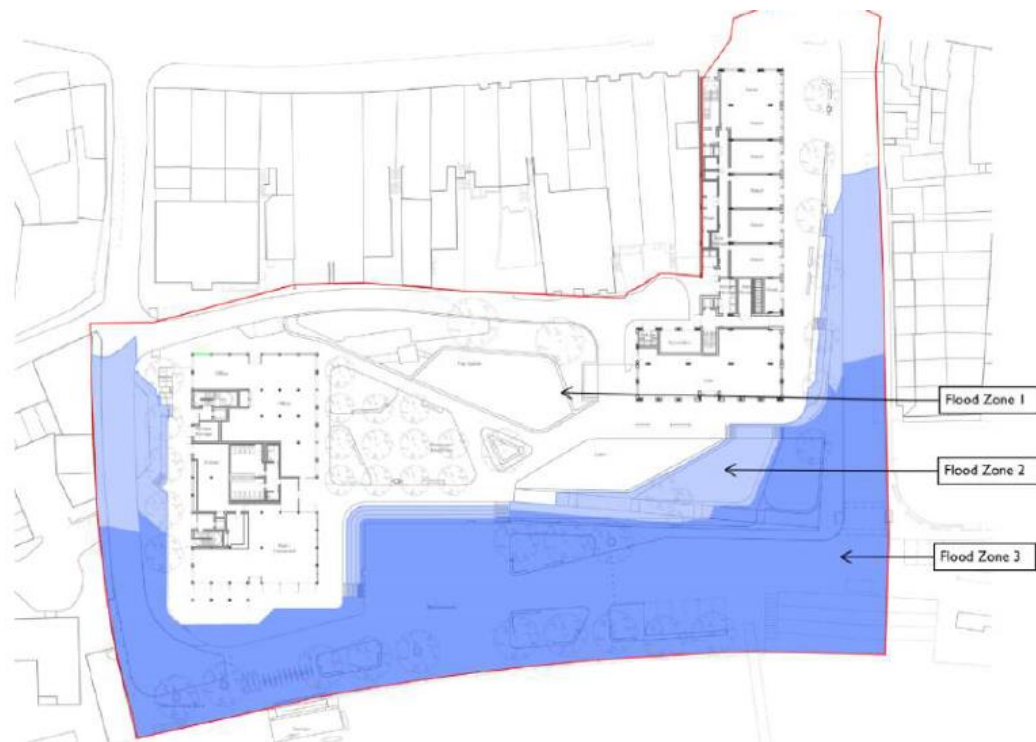
Figure 3: Flood Zone extents in the Proposed Development
