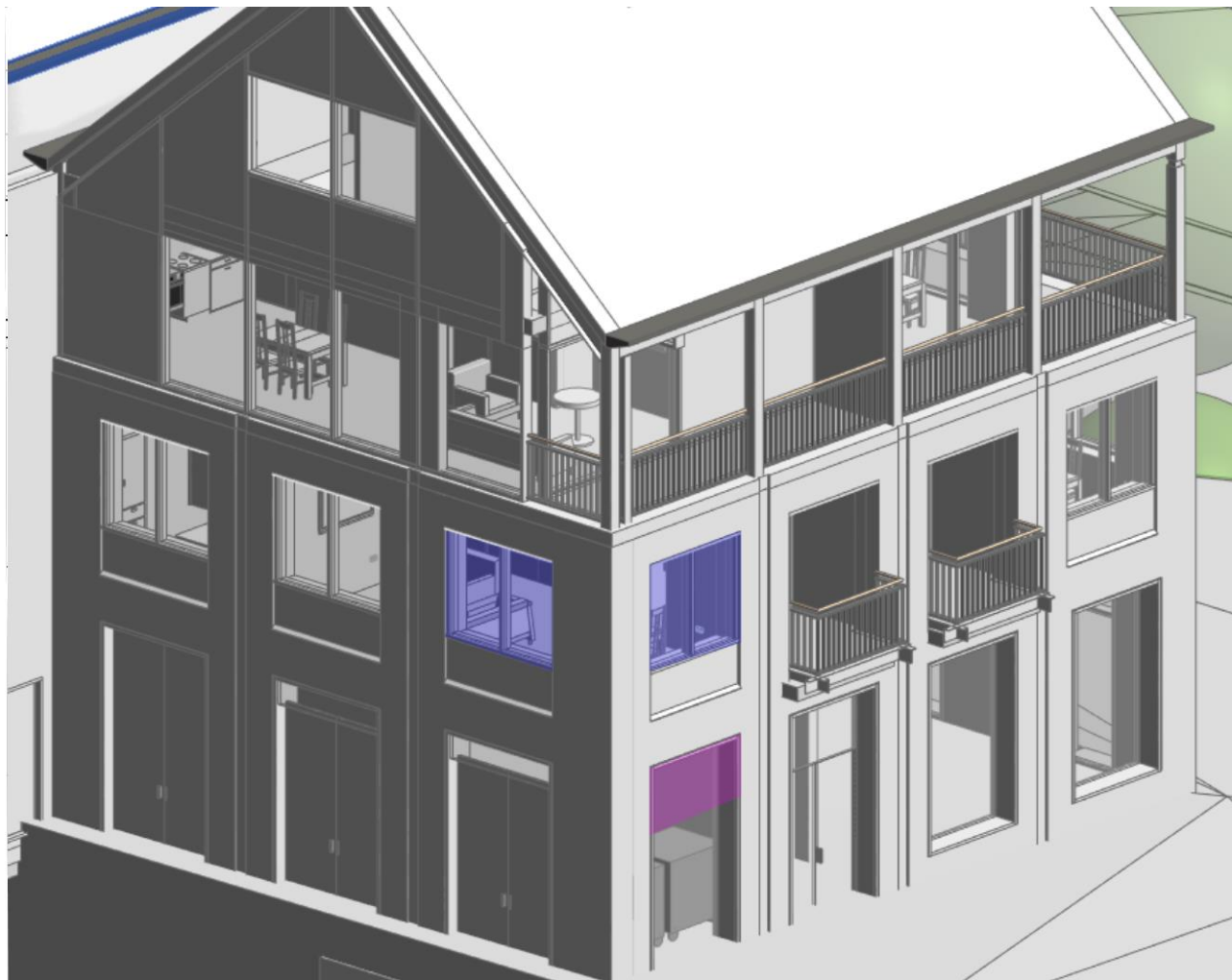
Figure 7: Kitchen exhaust location (shaded pink) and nearest sensitive receptor adjacency (shaded blue)
