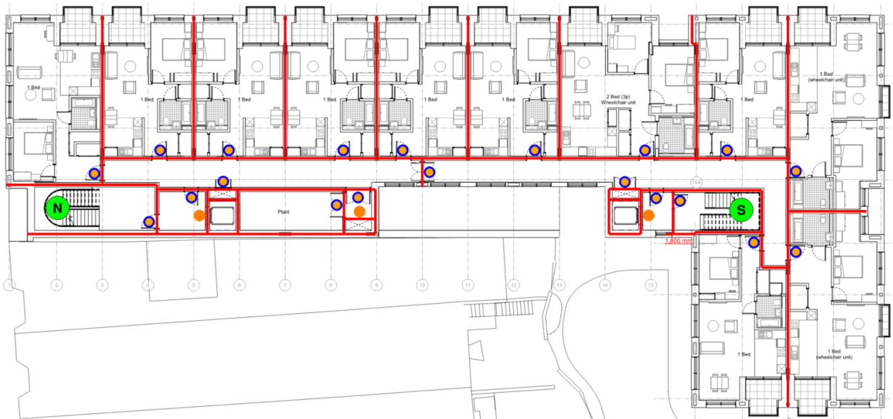
Figure 26 Water Lane typical upper floor residential compartmentation strategy
