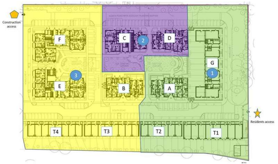
Figure 3.2 Indicative Construction Phasing
