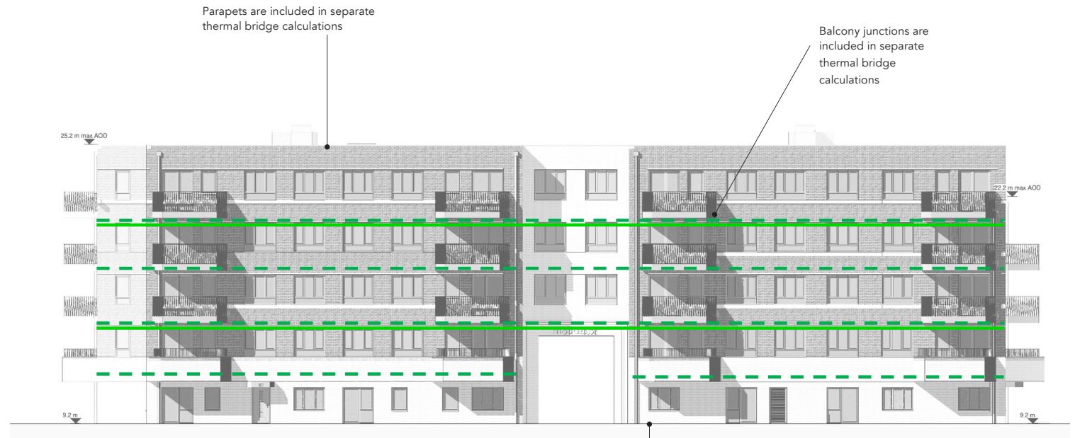
Heat losses via perimeter slab are included in separate thermal bridge calculations
