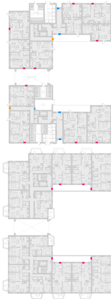
Ground floor plan and Typical floor plan with external doors to be fully insulated highlighted
