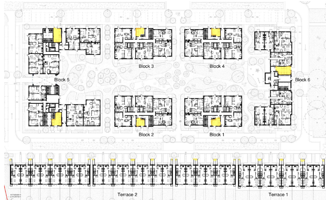
Ground floor plan highlighting provision for operational waste
