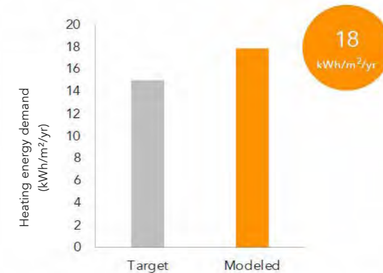
Total heating energy demand of building compared to the Passivhaus target of 15 kWh/m 2 /yr
