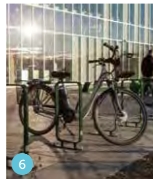
Furniture type 6 Powder-coated steel cycle stand (2 cycles per stand)
