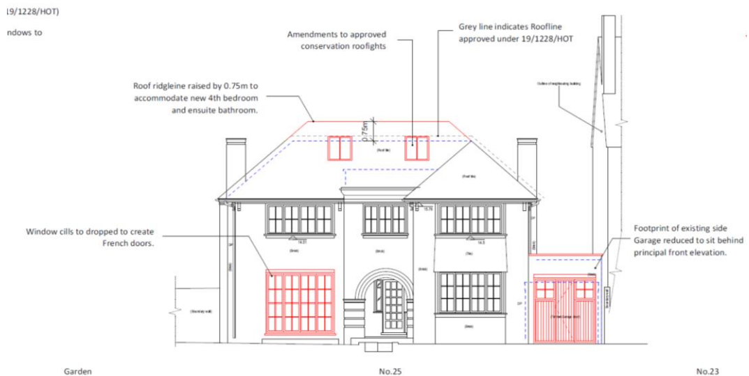
Figure 14: Proposed front elevation showing the wholly minor increase in ridge height at the application site
