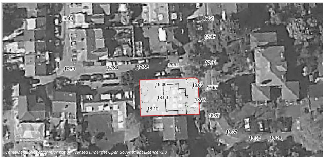
Figure 3: Ground elevations - extracted from 1m resolution LiDAR data
