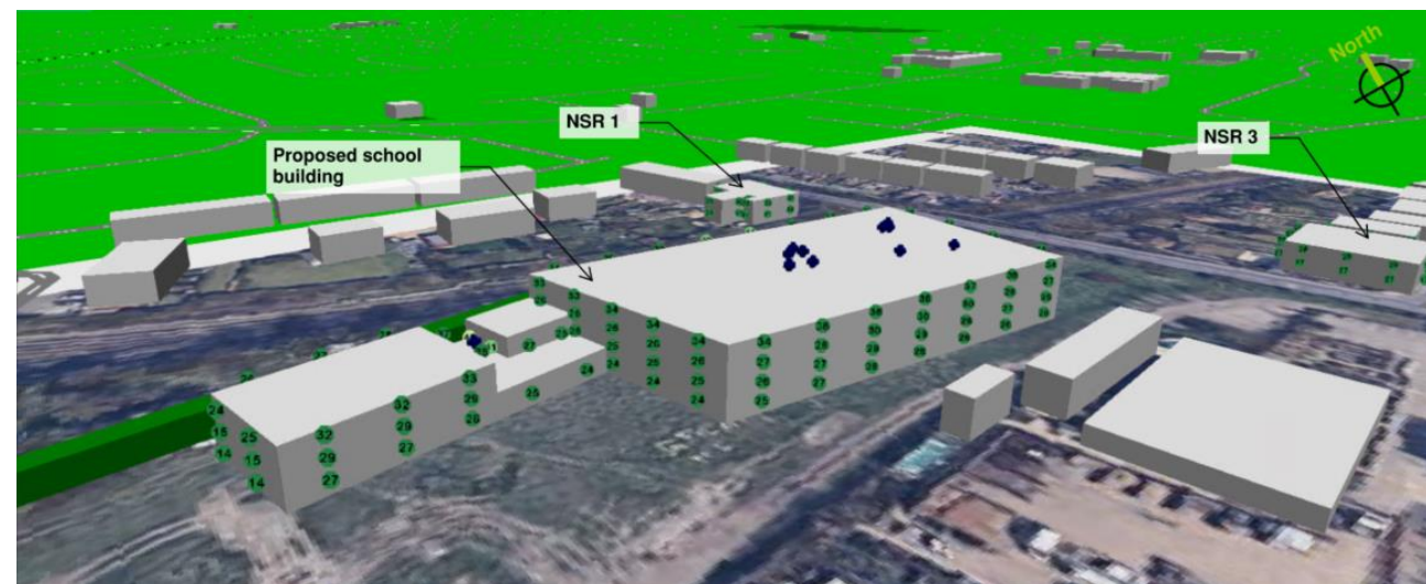
Figure 5—1 Image of model showing highest predicted L_{Aeq,T} (dB) noise levels at the proposed façades and NSR 1 and NSR 3 façades from proposed plant during school hours (07:00 to 19:00 hours)
