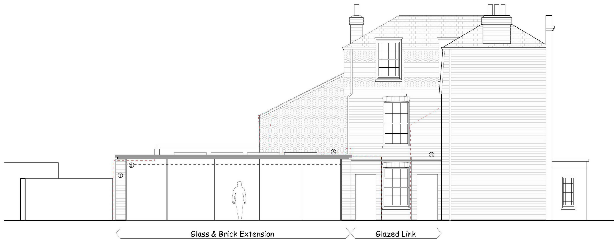
Proposed Side Elevation - Showing Glass Link
