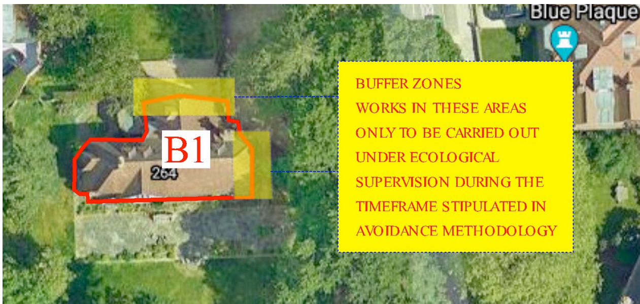
Figure 7: buffer zones indicating where works are time-restricted to ensure bat roost is not adversely impacted
