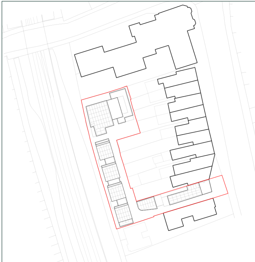
Figure 4 –Available roof space at the Proposed Development –area available for PV highlighted in red (MAA Architects)
