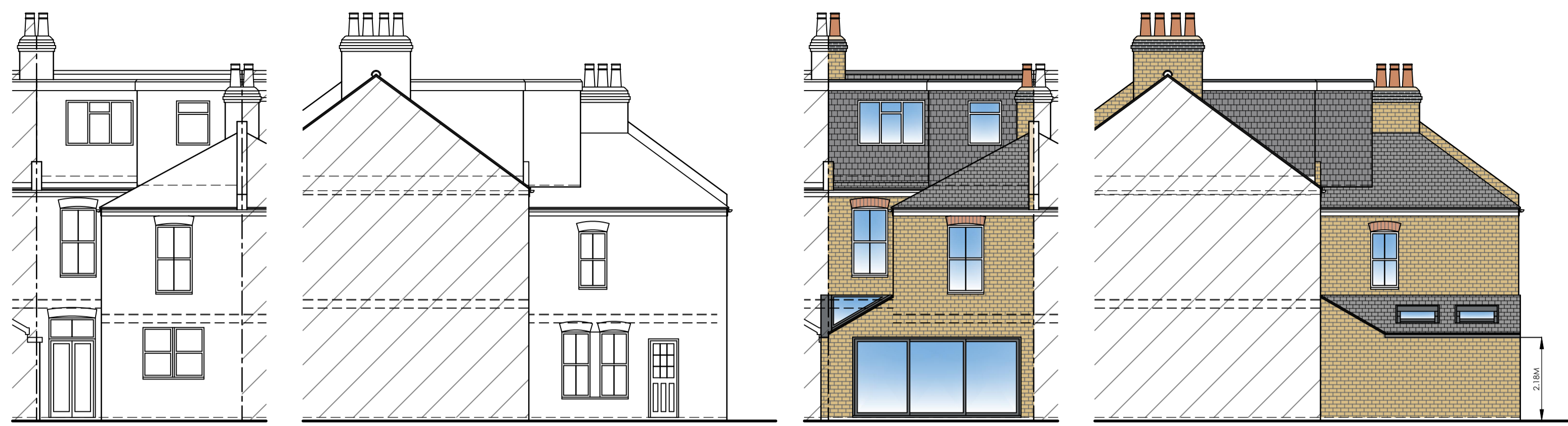
EXISTING REAR ELEVATION 1:100 EXISTING SIDE ELEVATION 1:100 PROPOSED REAR ELEVATION 1:100 PROPOSED SIDE ELEVATION 1:100
