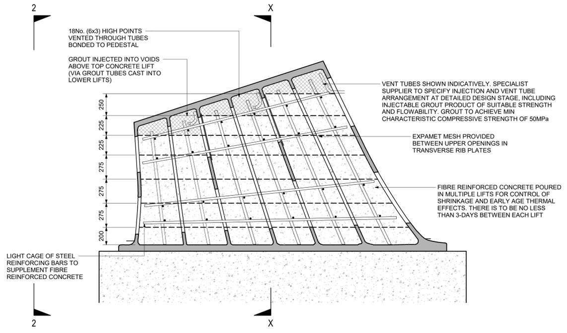
**CONCRETE PEDESTAL INFILL SECTION**
