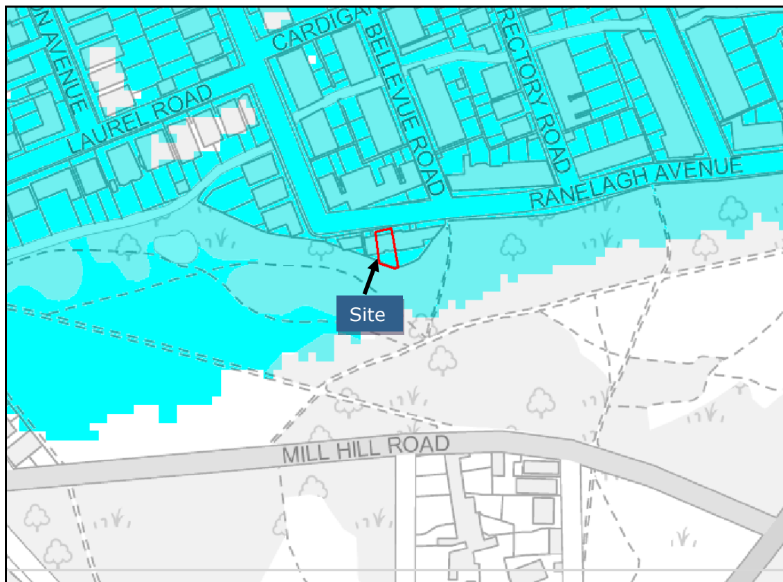
Figure 5: Breach inundation map for 2100 (taken from Thames_Upriver_Breach_Model_P6)
