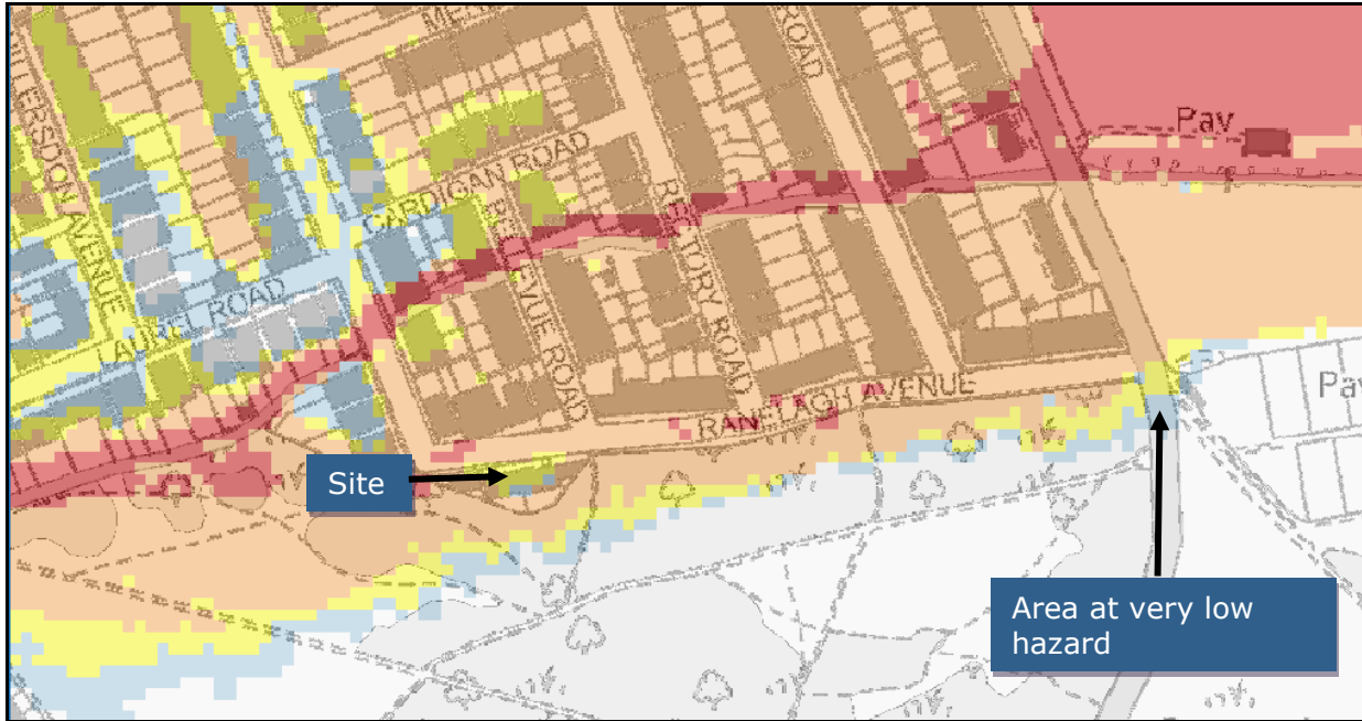
Figure 8: Breach hazard map for 2100 (taken from Thames_Upriver_Breach_Model_P6) (refer to Table 3 above for classification)
