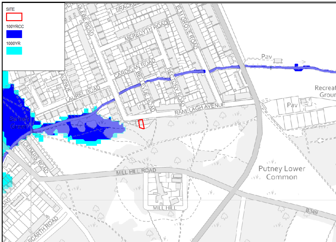
Figure 6: Flood extents from Beverley Brook (taken from Beverley Brook 2009 model)
