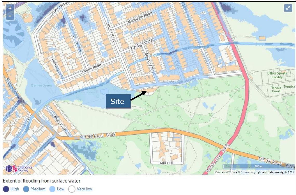
Figure 9: Environment Agency Surface Water Flooding Map (Source: Environment Agency, 2021)
