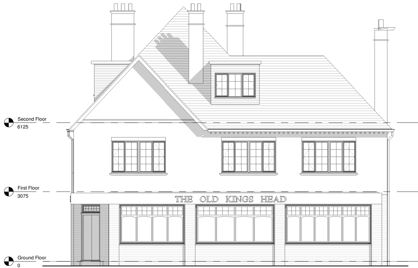
Existing North Elevation 1 : 50
