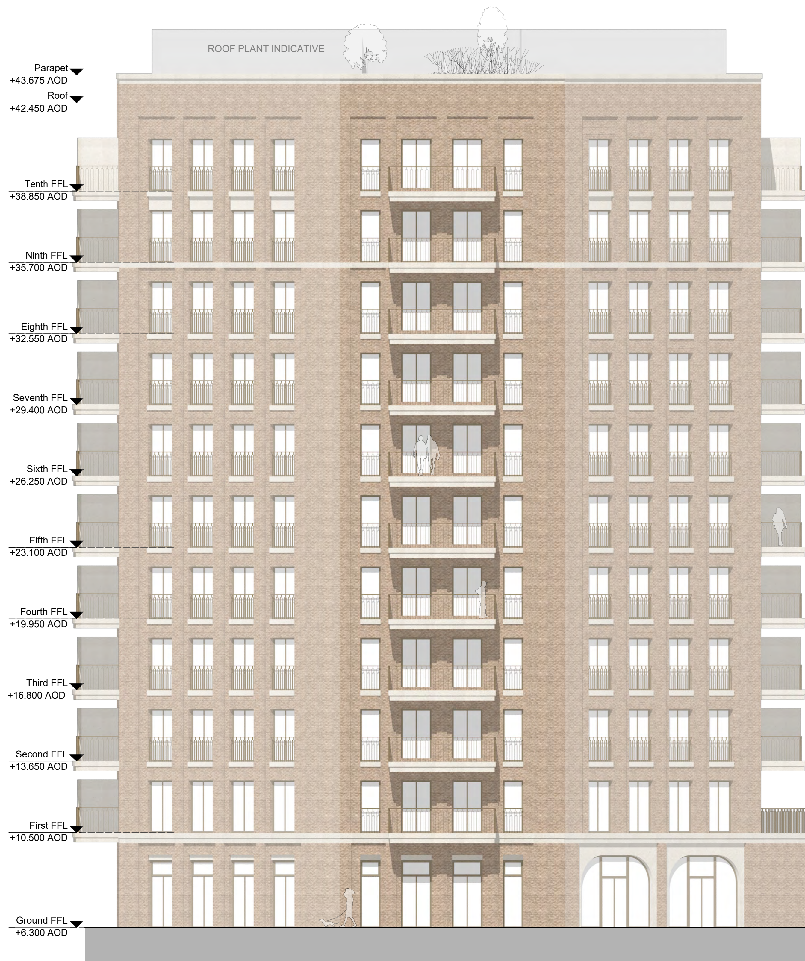
3 Block B South East Elevation Scale: 1:100
