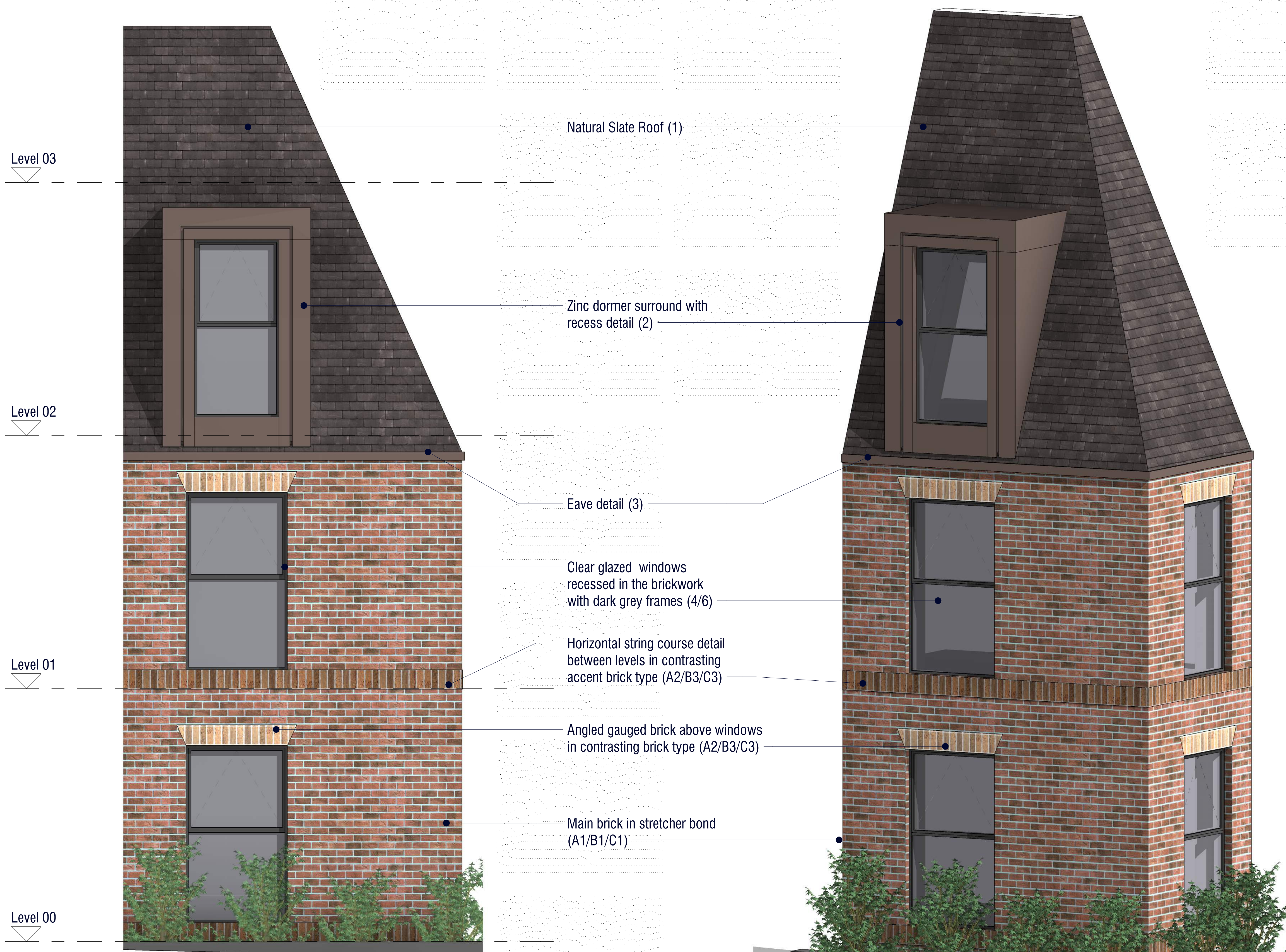
1 Typical Corner Condition Elevation 1 : 25
