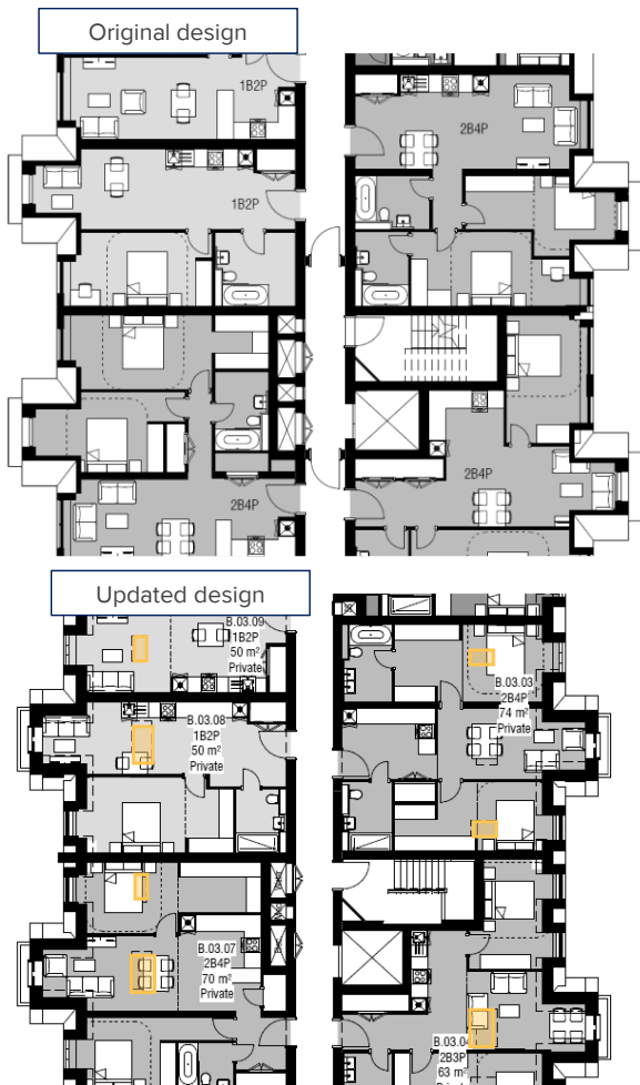
Figure 3: Demonstration of the addition of rooflight to deeper rooms at the top floors that are achieving lower ADF levels
