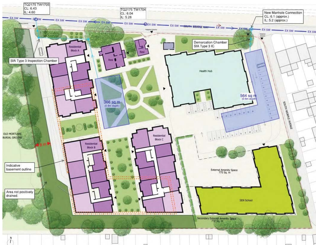
Figure 12: Proposed locations of geocellular surface water attenuation.
