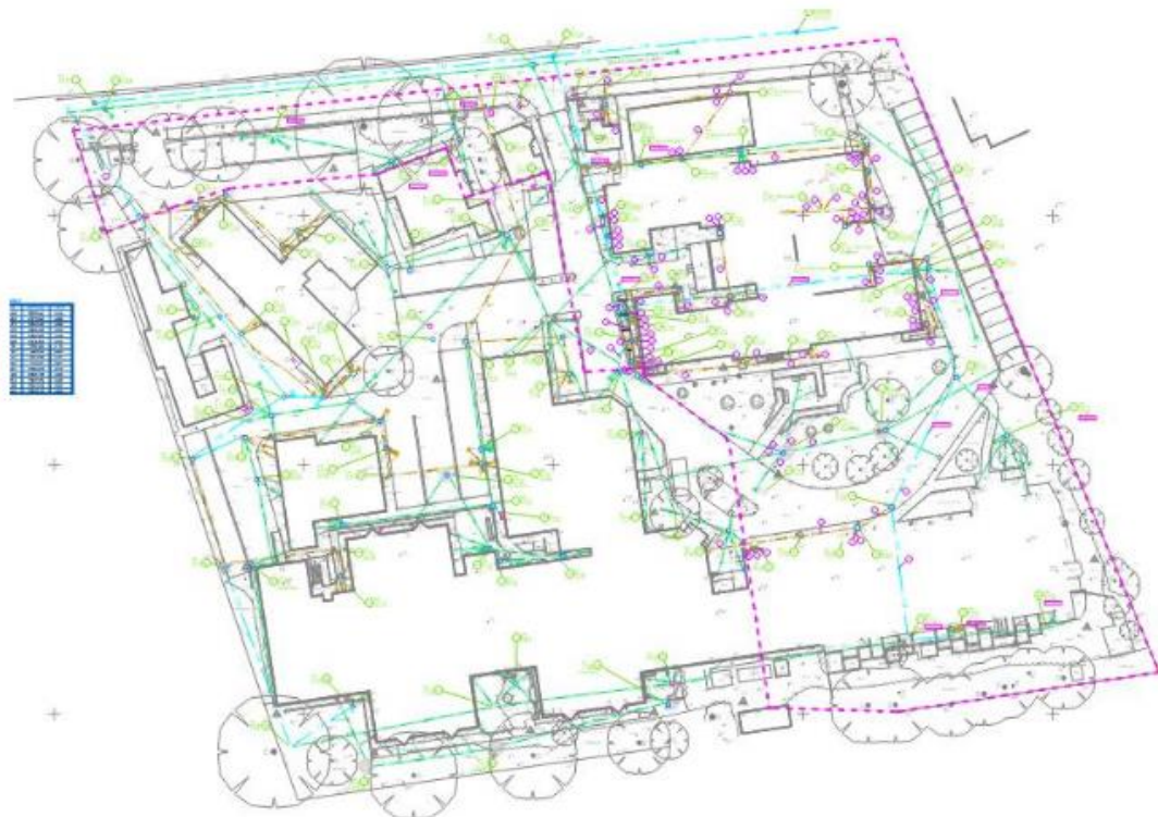
Figure 2-5: Existing drainage on site (in purple)
