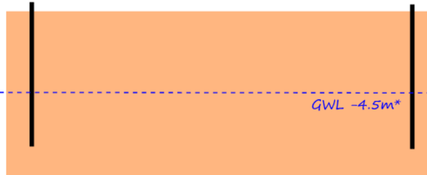
Stage 1: Install wells and dewater construction site
