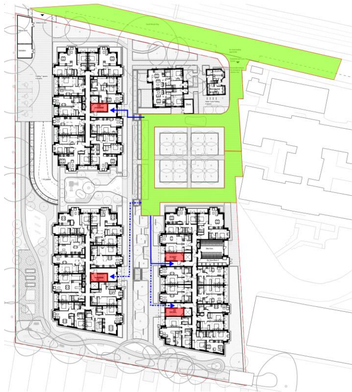
Figure 3: Site plan illustrating fire service vehicle access routes in green. Escape stairs are indicated in red, and firefighting access in blue.
