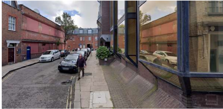
A : Castle Yard - west Repave widened footway to match existing with recessed service cover where possible. Retain granite kerbs. Careful consideration of ramp, levels, gradient and potential balustrade, reintervention on public realm.
