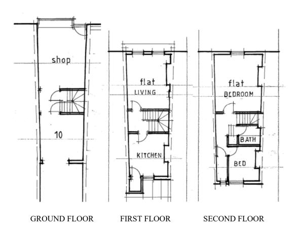
Planning approval is sought for creating a protective means of escape from the flat by reconfiguring the stairs and providing a fire lobby between the shop and the flat entrance.
