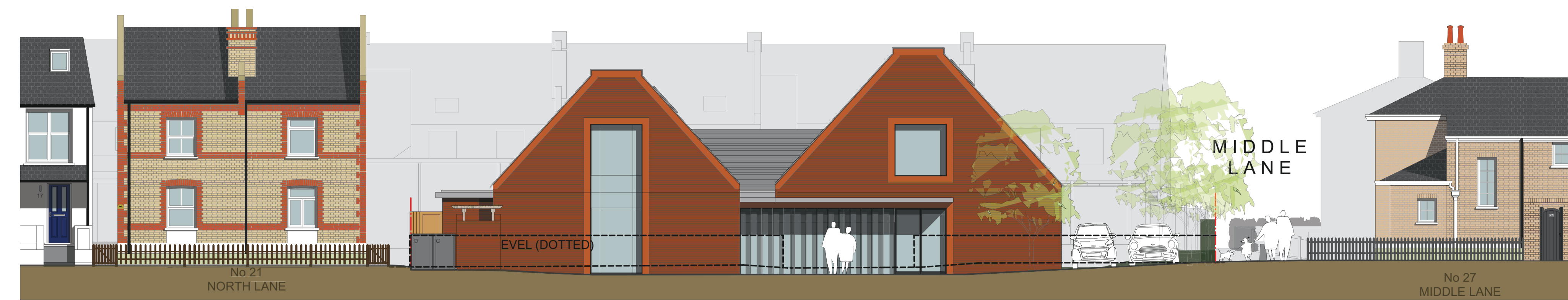
FRONT ELEVATION (WEST FACADE) 1:100
