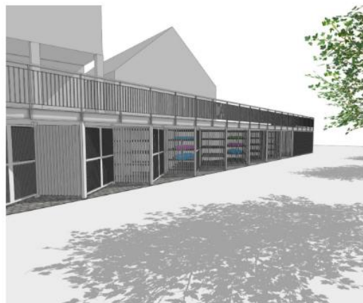
The doors to the individual boathouse sections have a lightly different façade treatment made up of PPC metal bars with gaps to allow water flow
