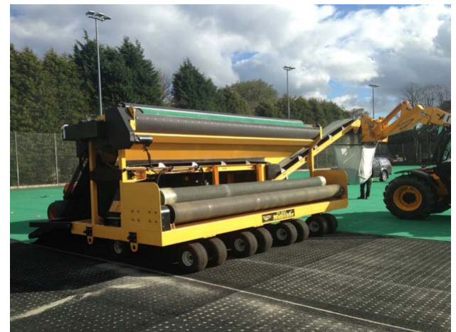
Automatic carpet lifting and rolling operation
