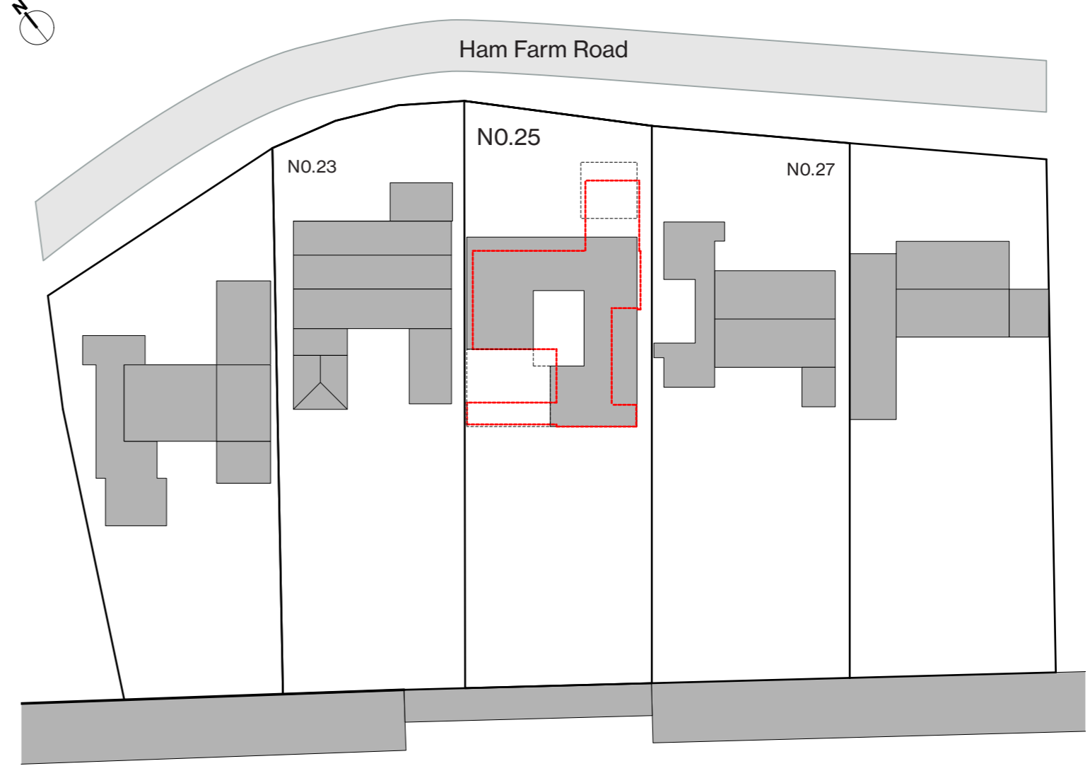
Plan Overlay of proposed footprint in relation to existing (existing house shown in red outline)
