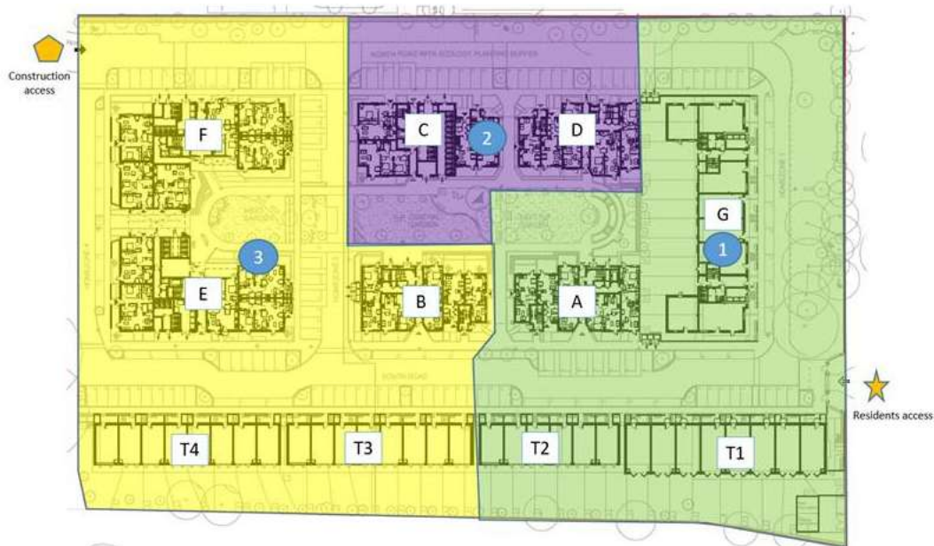
Figure 3.2 Indicative Construction Phasing
