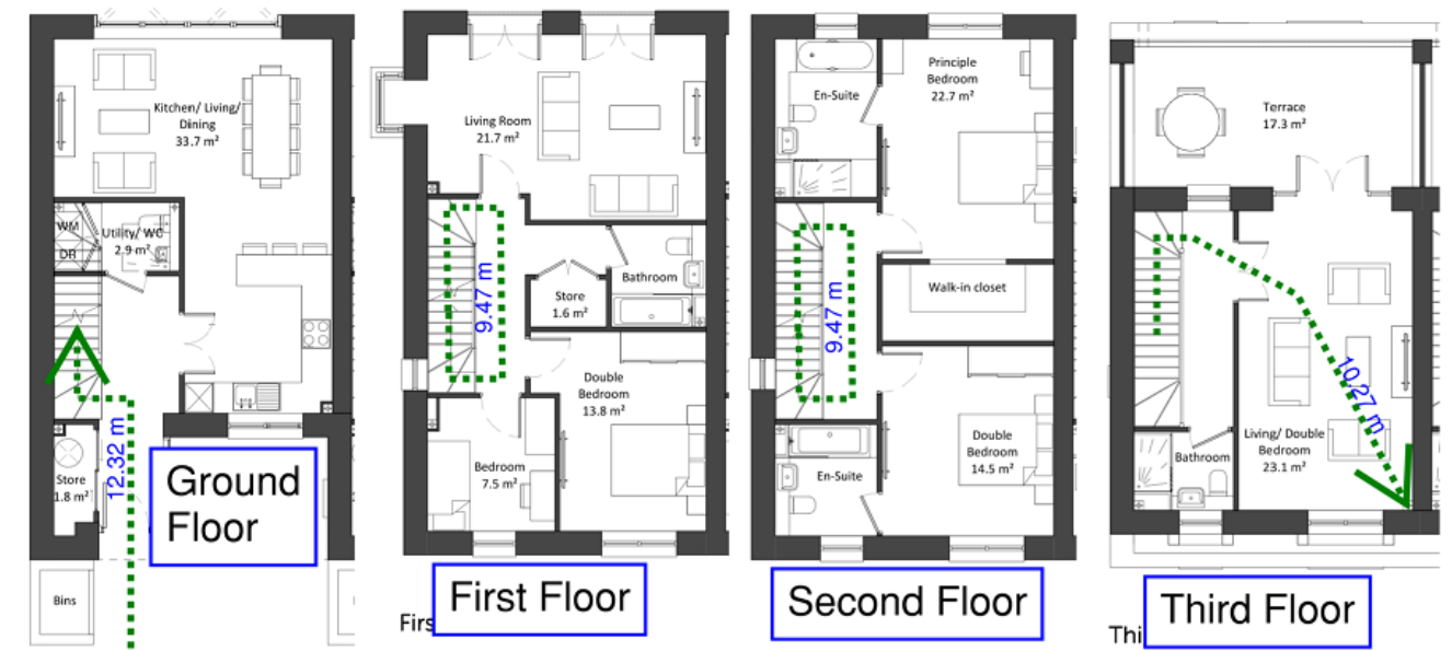
Figure 33: Hose Lay Distances - Townhouses
