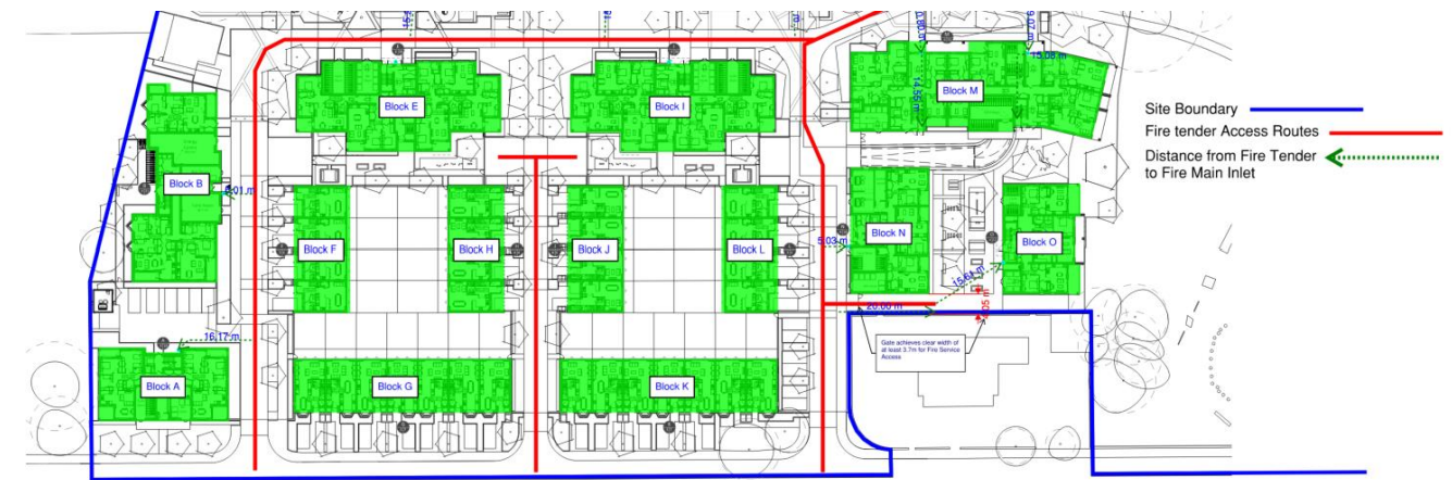
Figure 29: Fire Service Access – Part 1
