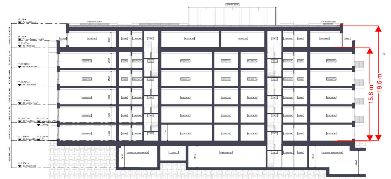
Figure 8: Building Heights - Block M
