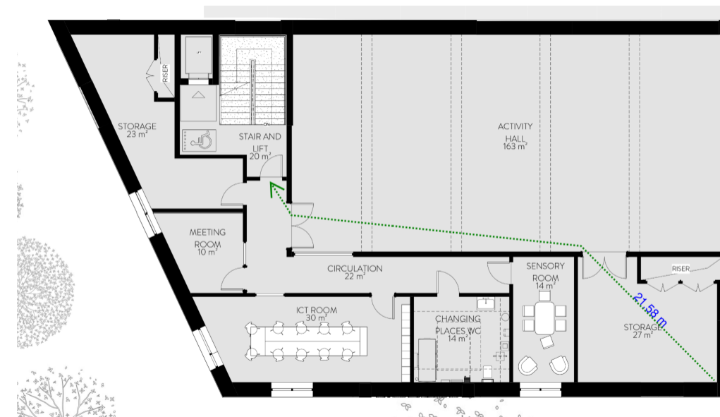
Figure 5: Travel Distances from Community Centre First Floor
