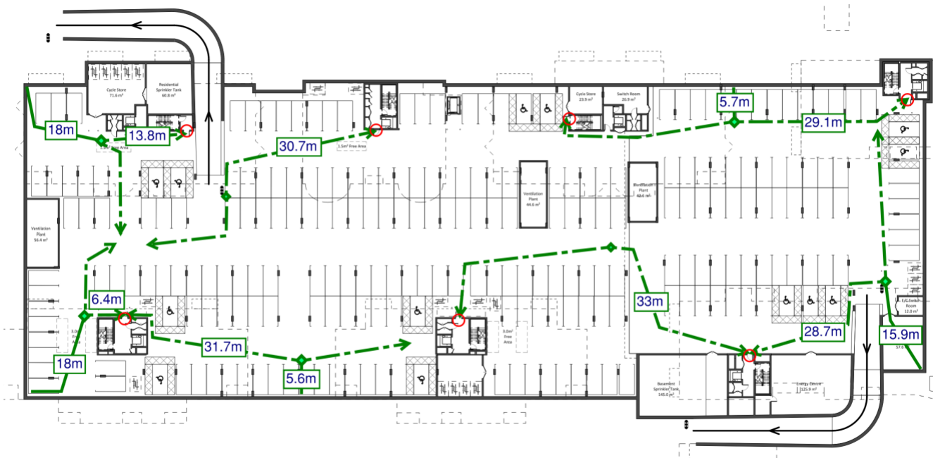
Figure 23: Means of Escape from Basement Ancillary Areas
