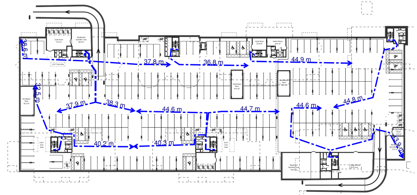
Figure 32: Hose Lay Distances - Basement Car Park
