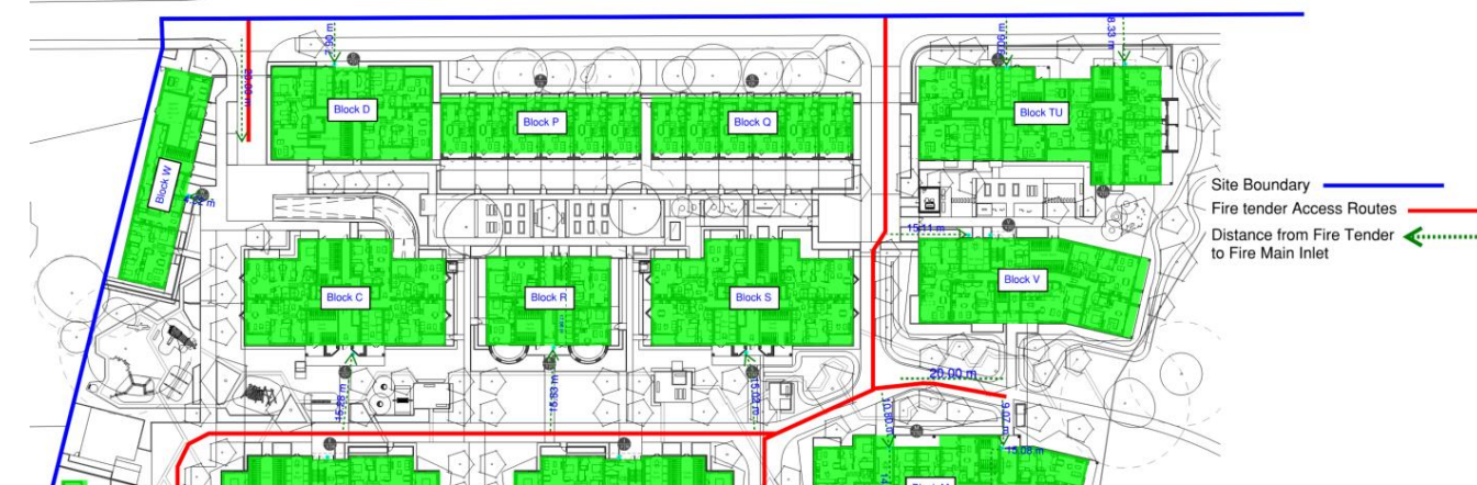
Figure 30: Fire Service Access – Part 2
