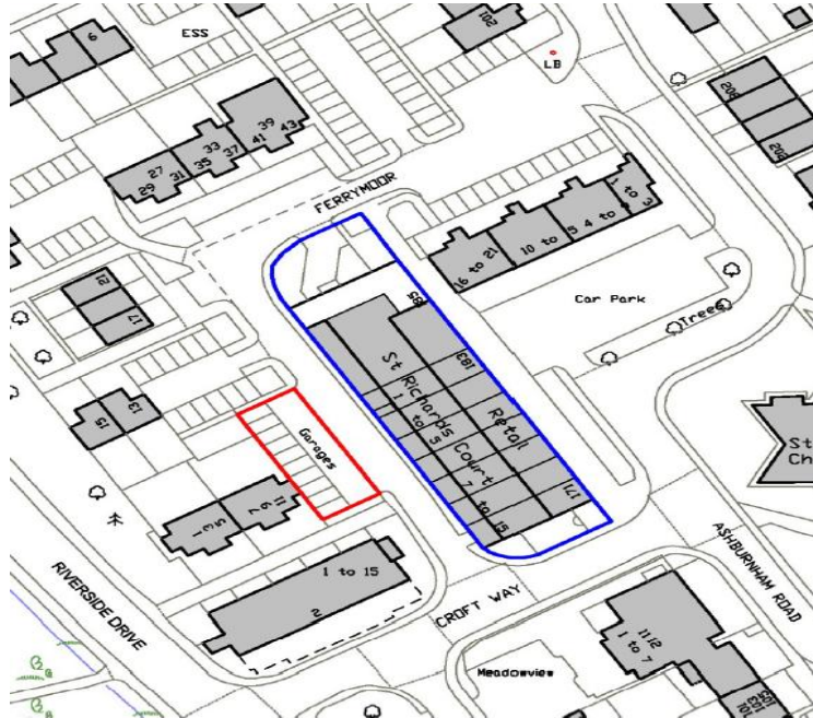
Diagram 1 showing Fire Service vehicle access from Riverside Drive & Croft Way to Ferrymoor. The red rectangle shows the location of the new Development. (Taken from Report Ferrymoor Ham site 2 Garages, Design & access statement 10 February 2022: Rev. A)
